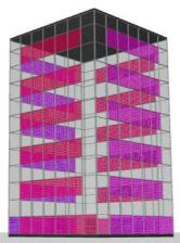
Fig. 1. Arrangement of integrated PV panels on cubic form
